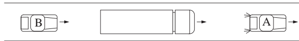
Figure 4.1: Extended Electronic Brake Lights: Vehicle A is braking, but vehicle B is not aware of the hazardous situation ahead as its line of sight is blocked by the truck. Safety can be improved if vehicle A broadcasts a warning message.
