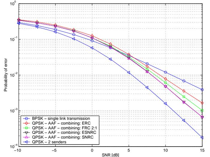
Fig. 1. The different combining types are compared with each other. The best performance results when using SNRC/ESNRC.
