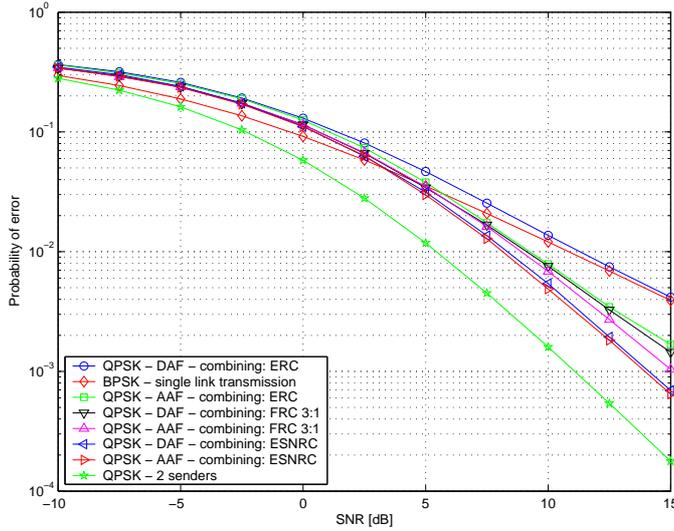
Fig. 2. The two diversity protocols (AAF and DAF) are compared with each other. Notice the different (optimal) FRC-ratios using either AAF or DAF.
