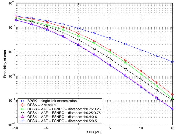
Fig. 3. A big benefit results when the relay is located between the sender and the destination.
