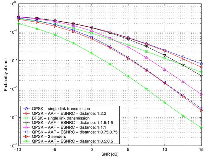
Fig. 4. Shows the effect of increasing the distance of the relay to the sender and the destination.
